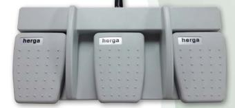
The 6226-0026 is a 3 pedal footswitch supplied with all grey pedals and base. With N/O contacts, the switch is supplied with 2 metre cable with free wire ends. It has IPX8 rating and is designed for operation at 24 V AC/DC.
