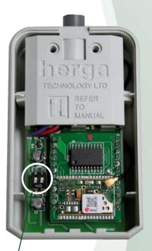
Removing the rear panel gives the user access to switches for setting the latency of the system and sleep timeout of the connected transmitters
