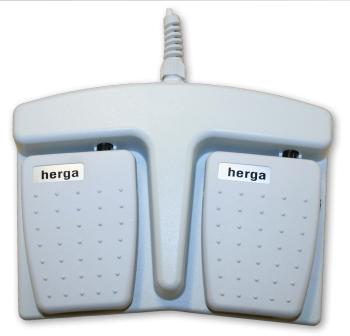
The Herga USB footswtch is programmed by the user to simulate up to three simultaneous keystrokes. No software installation is required as it will be recognised by the operating system once plugged into a USB socket. Programming is done simply by setting small switches inside the footswitch after having removed the cover (see pages 2 and 3).
