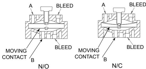
Where temperature compensation is required, consider carefully which side of the moving contact the bleed should be fitted. This will vary dependant on pressure or vacuum operation.
