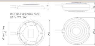
Note: To remove mounting ring from bellows as supplied, insert a 3 mm dia. bar in one of the holes & twist anti-clockwise through 41°. Mounting ring can be used as a template for drilling/tapping holes in mounting face.
